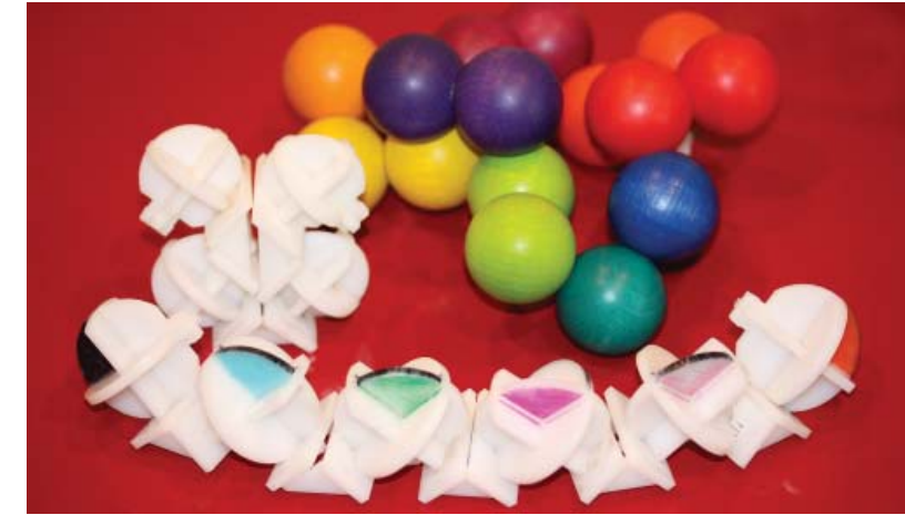
Fig 2 Header pin and socket modules which connect to mimic modular toy by beyond123. Allows 360^\circ , planar rotation between adjacent modules.
