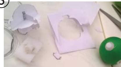
Fig 2. The final 3D module consisted of two cross header pins per module that could link with corresponding sockets. Paper prototypes of the 3D module were created initially to determine the geometry of each planar piece.
