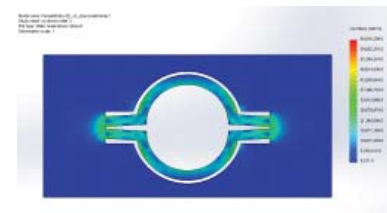
Fig 2 Analysis of design without circular cutout shows greater stress build-up.
