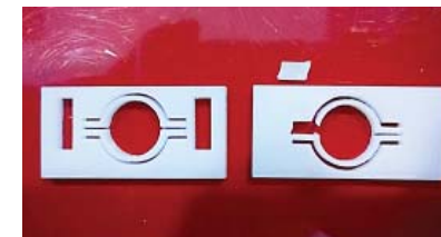
Fig 2 Failure of design in axial loading
