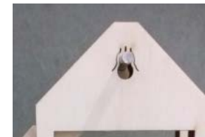
Fig 3 Inspiration for compliant stress relief components from "The Trebuchette" by E&M Labs.
