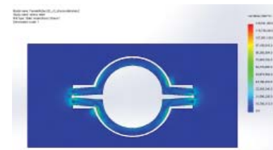
Fig 2 Analysis of design with circular cutout shows reduced stress build-up.
